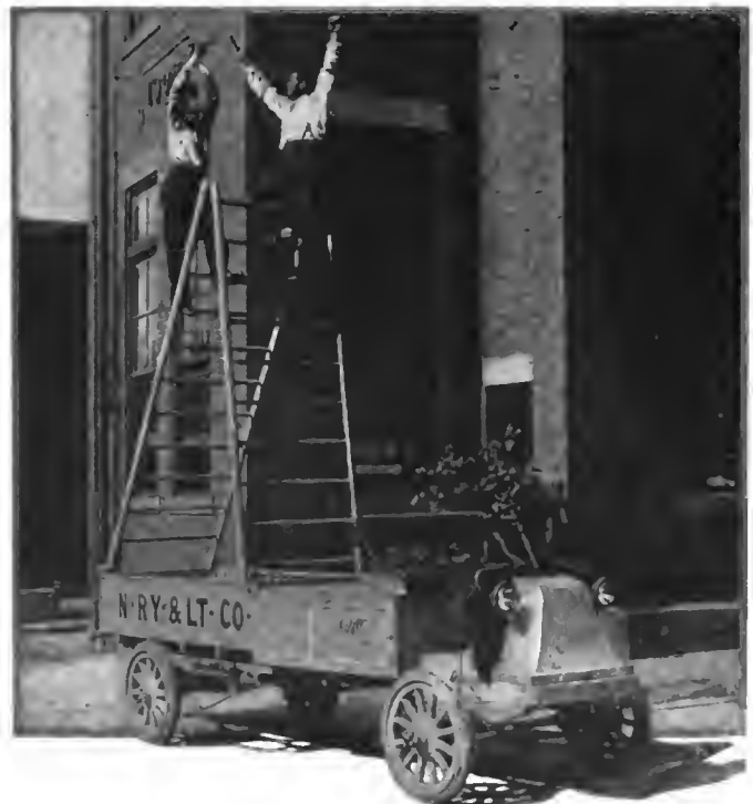
It is in emergencies that motor vehicles are at their best, and this fact has led many street railway companies to adopt the commercial vehicle for emergency wagons. The G. M. C. electric machine shown in the illustration is used in this capacity by the Nashville Railway & Light Co., Nashville, Tenn., and has shown much greater economy and efficiency than could be obtained with a horse-drawn wagon.
